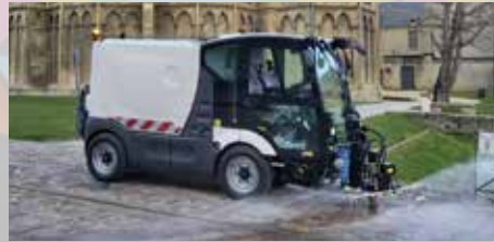
R2w The R2w is a dedicated washing solution with a large water tank and fixed spray bar for cleaning urban areas.
