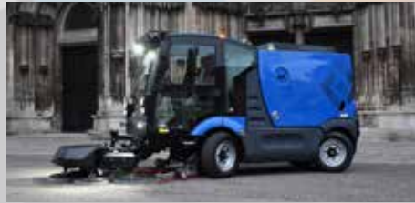
R2s The R2s is a dedicated road scrubbing machine, with 5 fixed scrubbing heads, for cleaning the road surface.
